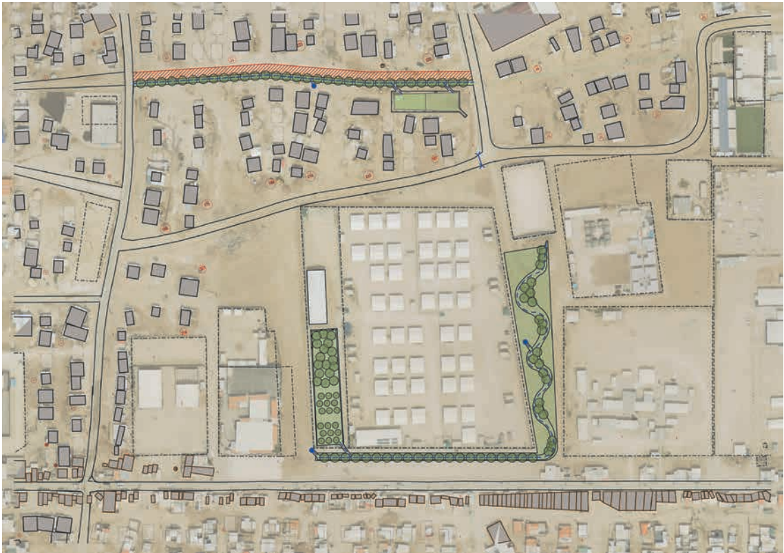
The design for the pilot location: avenues of eucalyptus help to slow down the runoff water from the hill. Along Jasmin Street green interventions help capture water, and create a central park with a school garden (below left) and a park zone (right).
